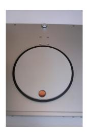
3 ) Turn the lid to the closed position and mount the stop knob back in place.
